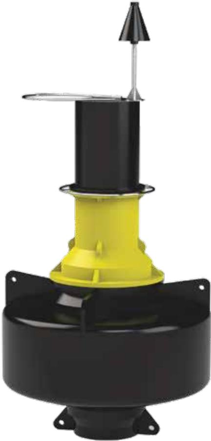
Tritonbuoys has developed a diverse selection of navigation buoys that adhere to rigorous quality standards and boast a proven track record of reliability. Each buoy is crafted from premium UV-stabilized virgin polyethylene and filled with closed-cell polyurethane to prevent water ingress if the outer layer is damaged. This design ensures exceptional performance and long-lasting durability.
